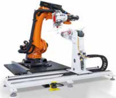
t bend – Fully electric mandrel bending machines
